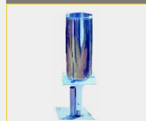
Standard precision instrument for the measurement of rainfall accumulation and/or rate. Contains an internal tipping bucket, designed for years of accurate and trouble-free operations.
