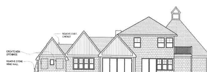
EXISTING/DEMO REAR ELEVATION SCALE 1/2" = 1'-0"
