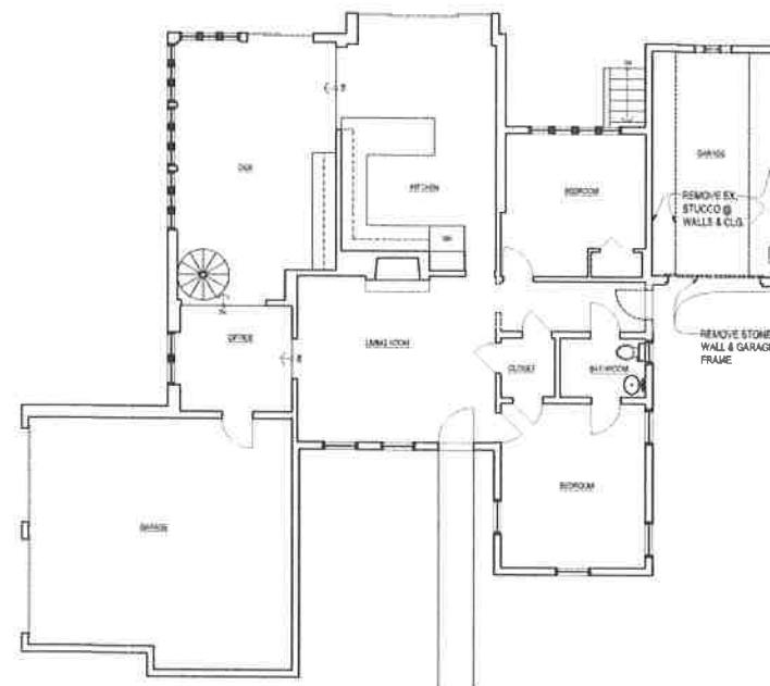
EXISTING/DEMO FIRST FLOOR PLAN SCALE 1/2" = 1'-0"
