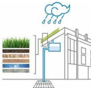
In addition to the landscaped terrace at the building entrance, Hunter Terrace will feature select areas of green roof to retain water and add insulation to the roof. Due to concerns over long term durability and maintenance, the development team will be selective in the areas to which green roofs are applied.
