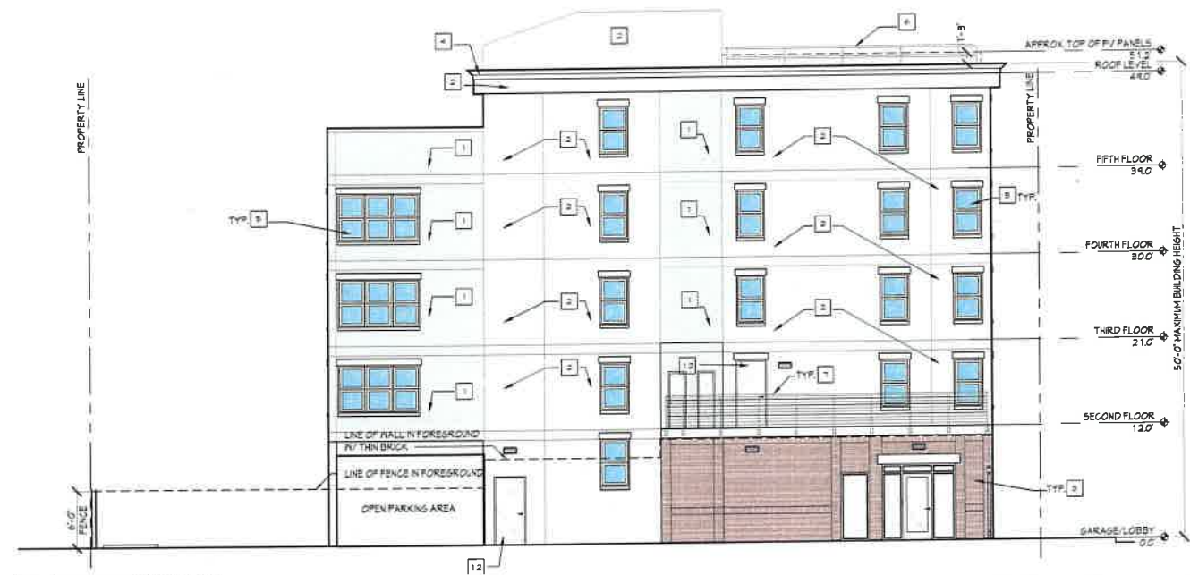
2 LEFT SIDE ELEVATION 1/8" = 1'-0"
