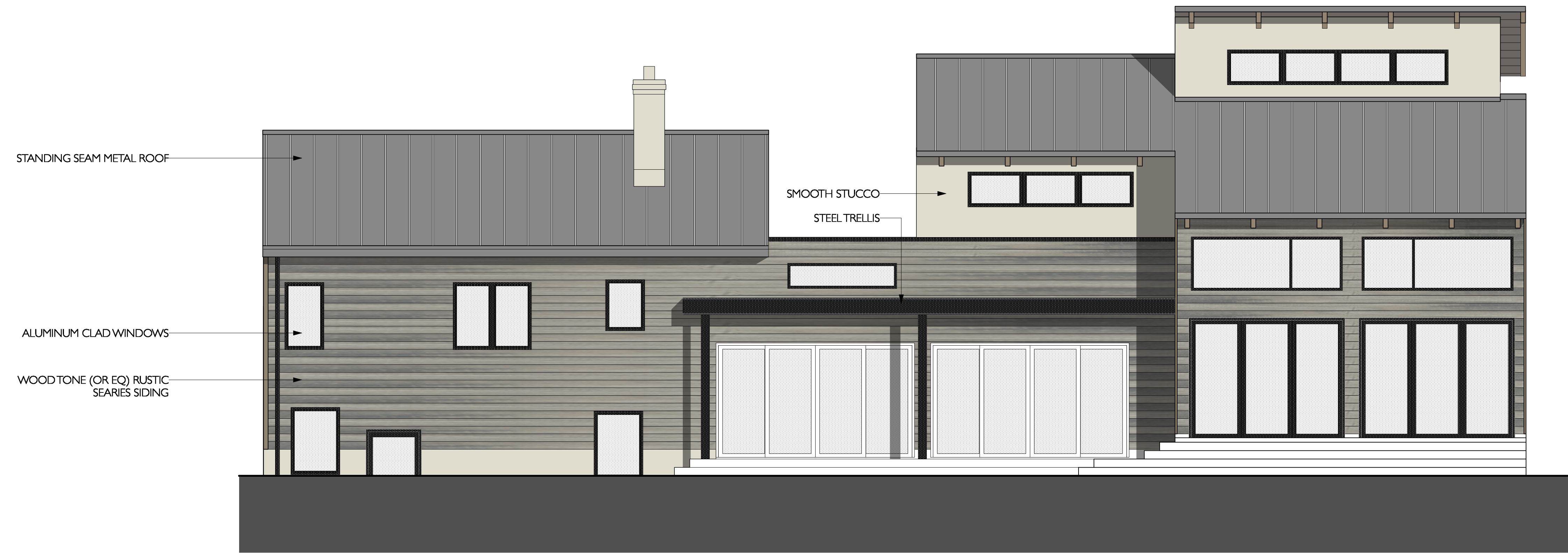
2 PROPOSED NORTH ELEVATION Scale: 1/4" = 1'-0"
