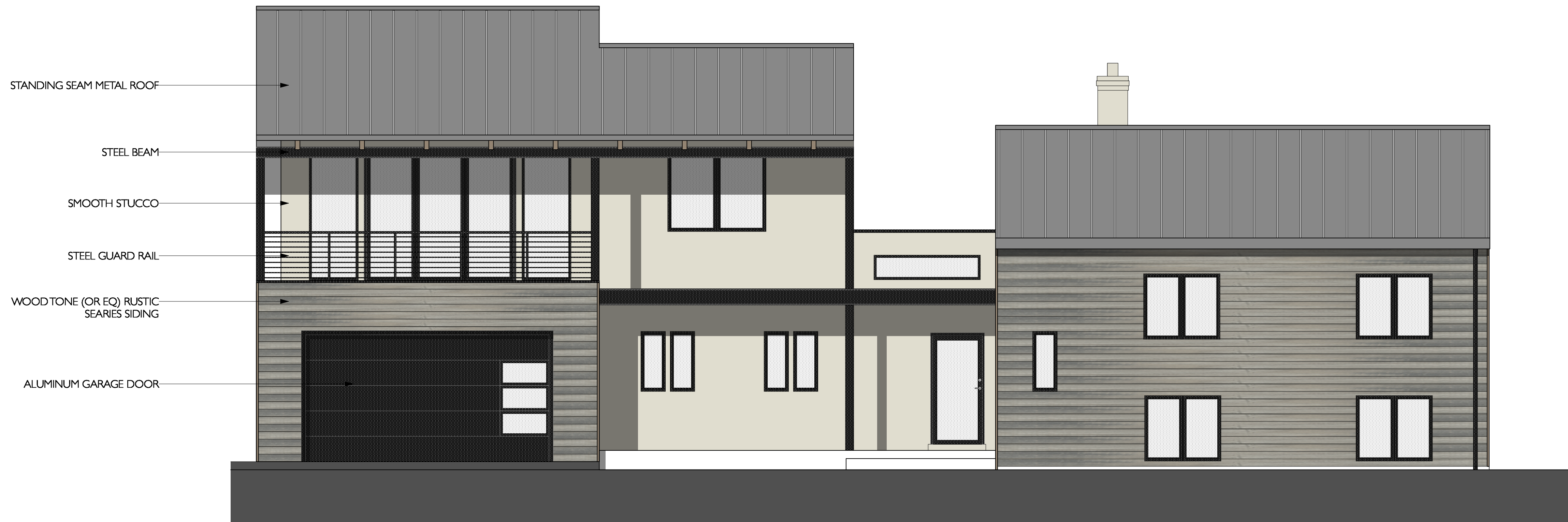
1 PROPOSED SOUTH ELEVATION Scale: 1/4" = 1'-0"
