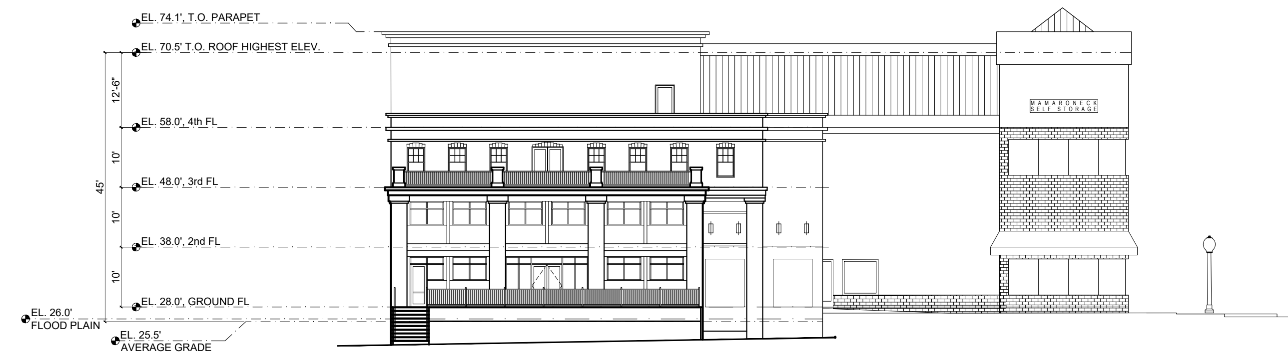
1 PROPOSED NORTH (FRONT) ELEVATION SCALE: 1/16"=1'-0"
