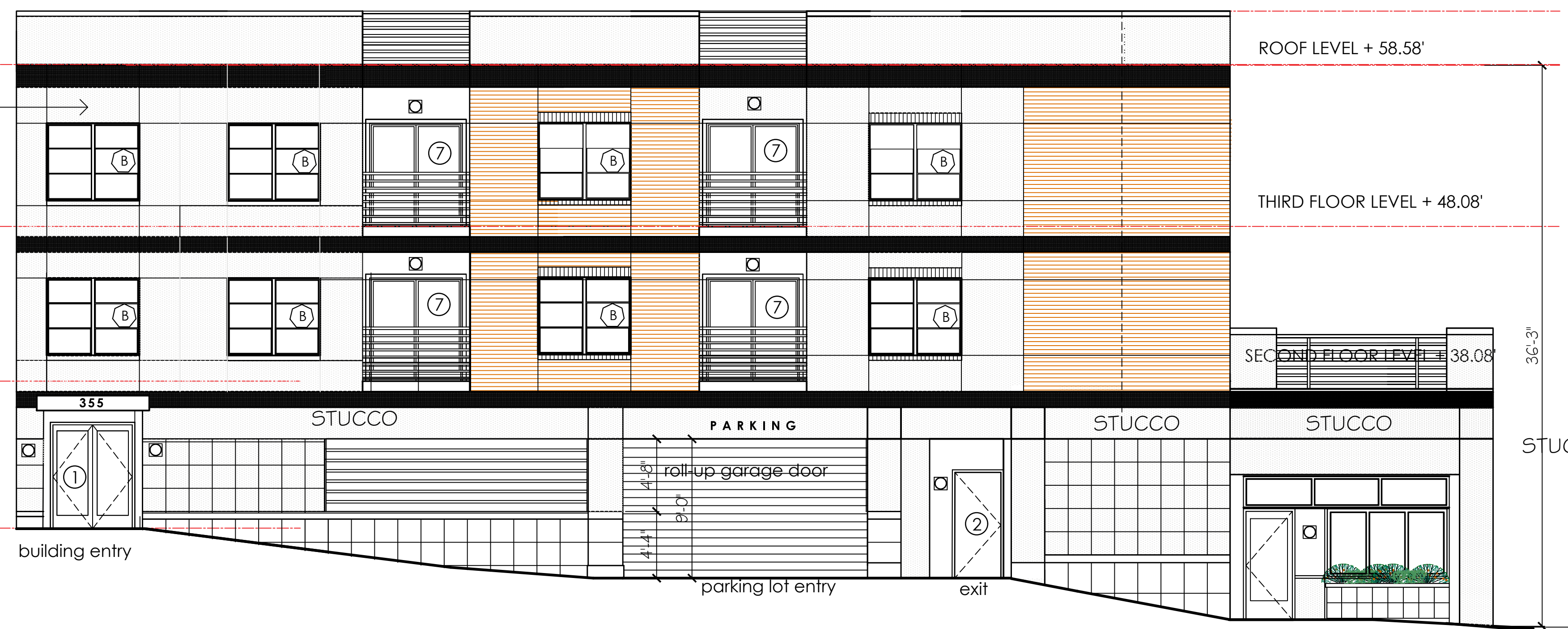
phillips park road elevation SCALE: 3/16" = 1'-0"
